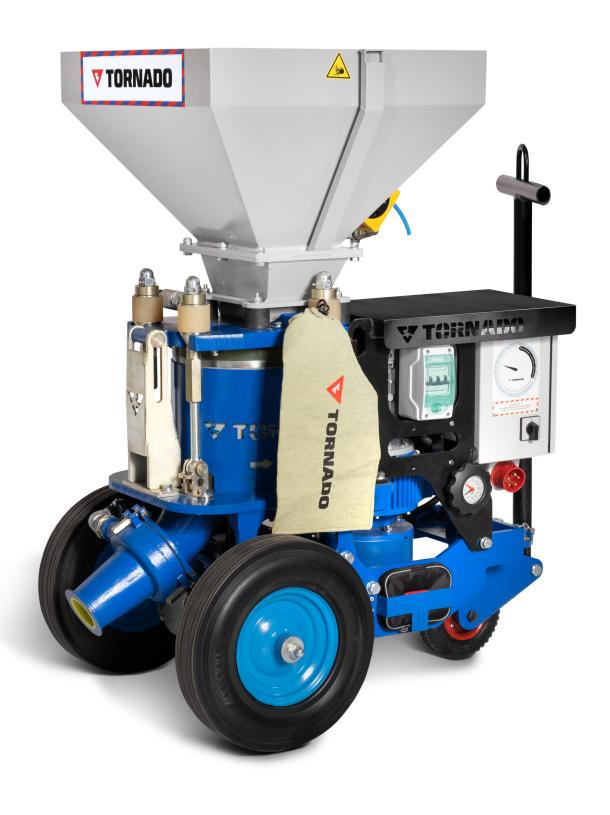
**Shotcrete** — is the construction technique, where concrete pneumatically conveyed through a hose and projected layer by layer at high velocity onto a surface
